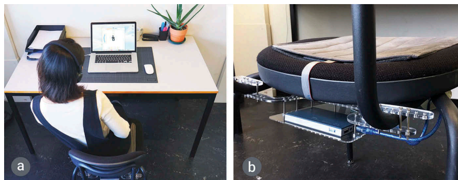
Figure 4. (a) The setup of the laboratory; (b) The HealthSit sit pad is mounted on the chair.
